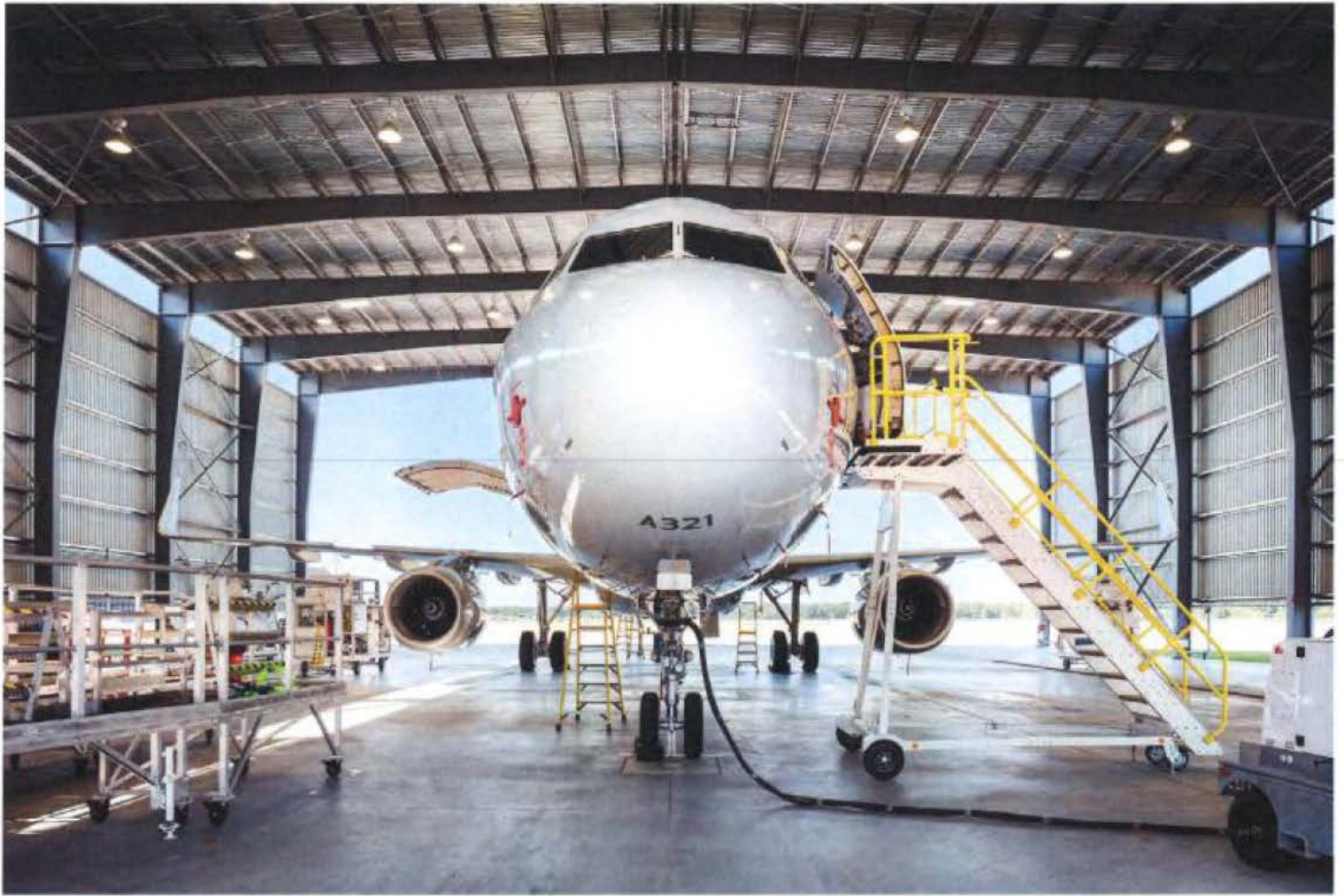
The completed A321, in the gauging canopy, where its fuel tanks are filled and tested. After a few more rounds of testing, its title will be transferred to American Airlines.
