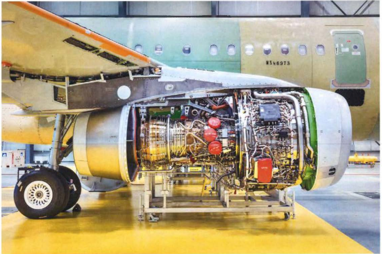
Each V2500 engine weighs approximately 5,250 pounds and generates 24,000 to 33,000 pounds of thrust at take off. Christopher Payne for The New York Times
