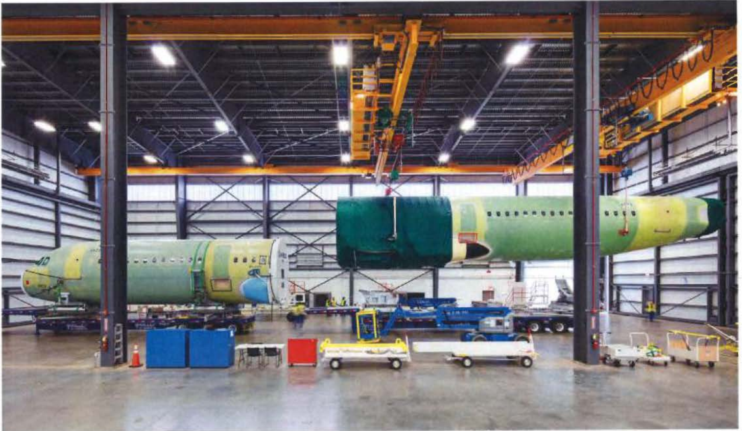
After arriving at the port in Mobile, all the major components are taken to the transshipment hangar, where they are inspected before going to the final assembly-line hangar. Here, the rear fuselage is lifted off a trailer. Times
