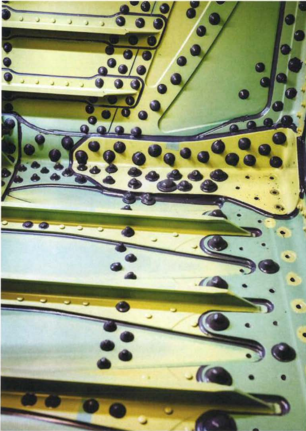
Each of the wings weighs 4.5 tons. Here, they are attached to the fuselage with approximately 1,200 rivets per side.
