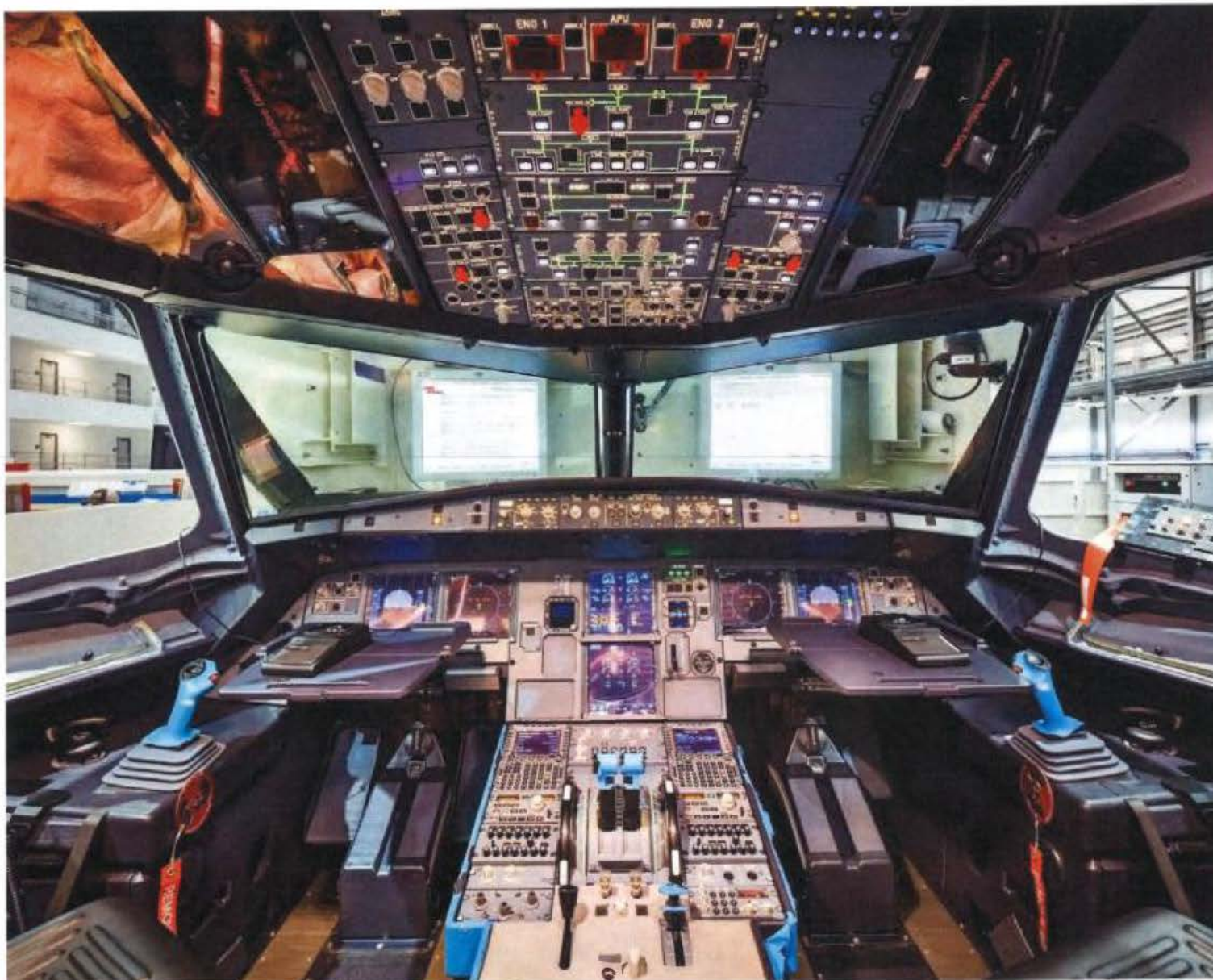
Inside the unfinished cockpit of the A321, which utilizes fly-by-wire controls.
