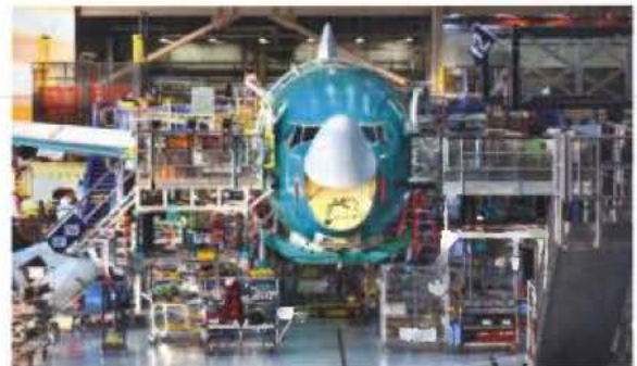
After finishing systems installation, a Boeing 737 is prepared for wing installation at Boeing's 737 assembly plant in Renton. (Mike Siegel / The Seattle Times)
