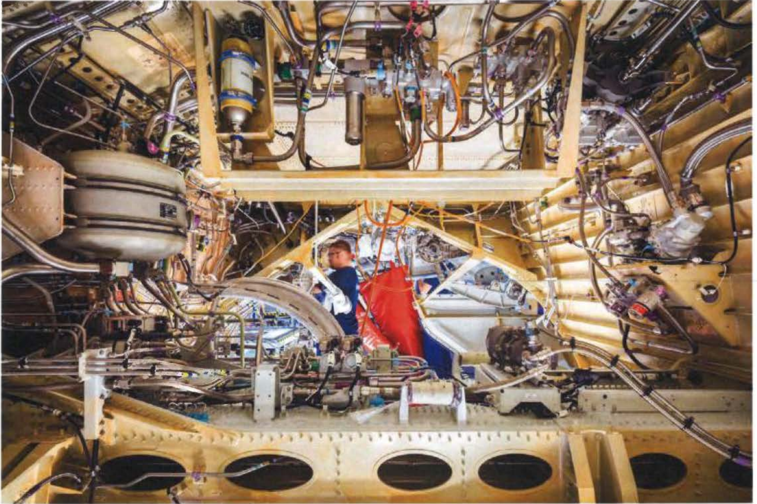
A look inside a main landing-gear wheel well. At this station, the aircraft is fitted with the vertical and horizontal stabilizers and the tail cone. This is also where the landing-gear doors, the radar and the navigation antenna are installed. Christopher Payne for The New York Times
