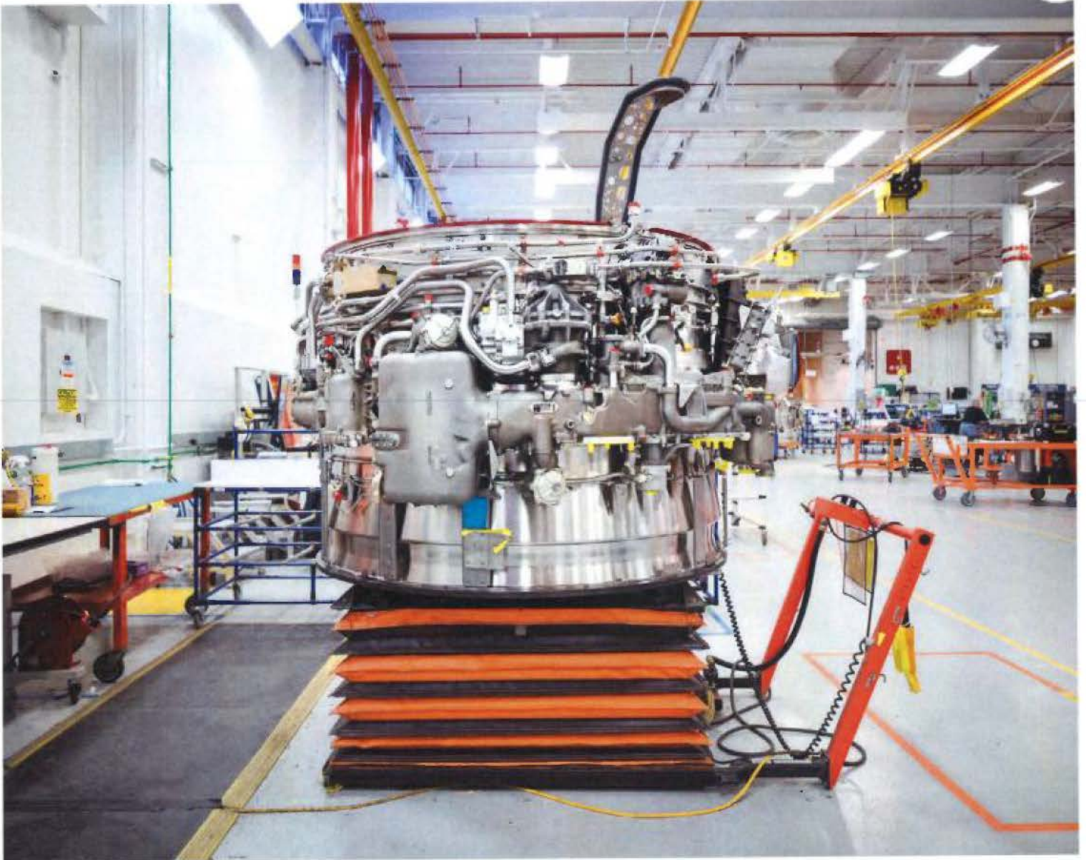
An engine for the A321 being built at the Pratt & Whitney factory in Middletown, Conn.
